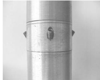
**NOTICE!** : The bracket can be placed and mounted in 4 positions in respect of the door. The mounting position can't be taken from the drawing, because there it is always drawn at 90° in respect of the door. The right mounting position can be taken from the calculation of strength. If this info is not available, then the position can be taken from the sticker on the delivered columns. If this says "NK"; "Free choice", then 180° or 0° is recommended.
